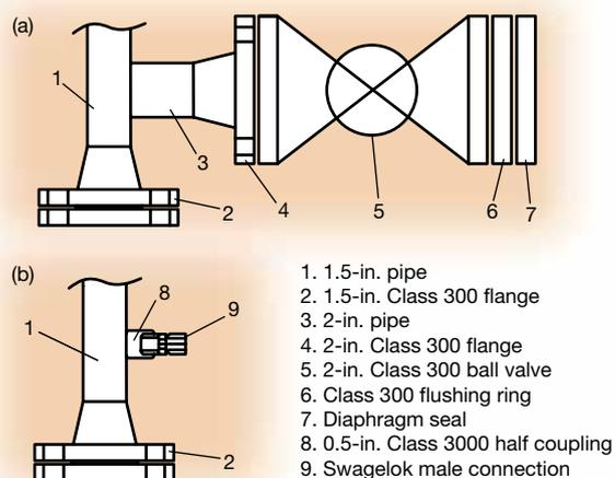
▲ **Figure 2.** (a) When piping specifications for a commercial plant are applied to measure differential pressure across a pilot-scale reactor, the incompatible piping creates a large dead volume that affects product quality and the ability to control temperature. (b) Replacing the entire assembly with a smaller-scale solution minimizes the dead volume and helps to control the reactor temperature profile.
