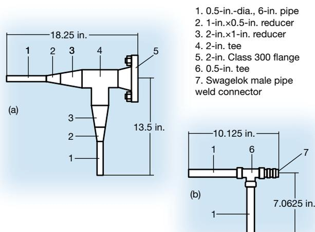
▲ **Figure 3.** (a) Large flanged thermowells introduce residence time issues in pilot plants, which have smaller piping. (b) Swaging the thermocouple directly into the process line is a more appropriate and scale-specific method of temperature measurement that lowers residence time because of the smaller volume.
